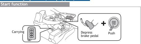
NOTE: Gear shift lever must be in Park and brake pedal depressed.
