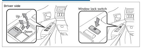
**Automatic operation (driver's window only)** Push the switch completely down or pull it completely up and release to fully open or close. To stop the window partway, operate the switch in the opposite direction.
